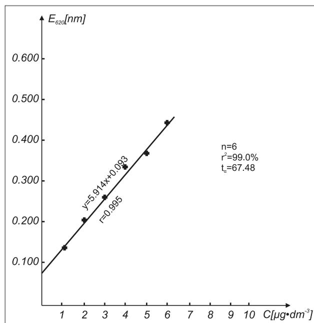
**Figure 2.** Calibration curve of indole concentration in 1 dm<sup>3</sup> of urine
