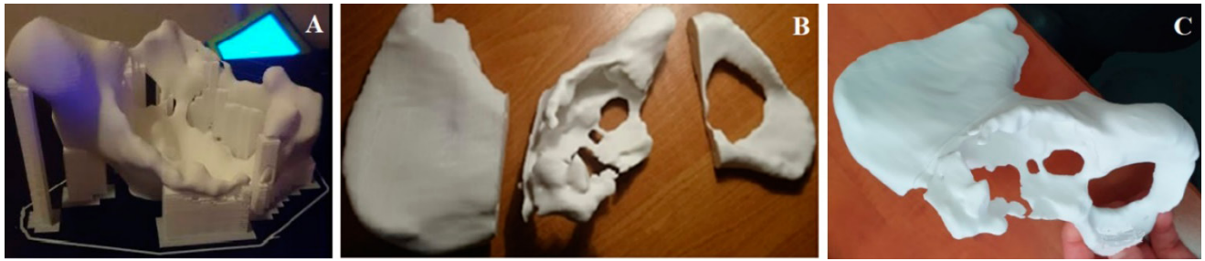
Figure 6. A-C, 3D prints of the pelvic bones. A – 1 of 3 parts with supports. B – 3 parts without supports. C – 3 parts connected together
