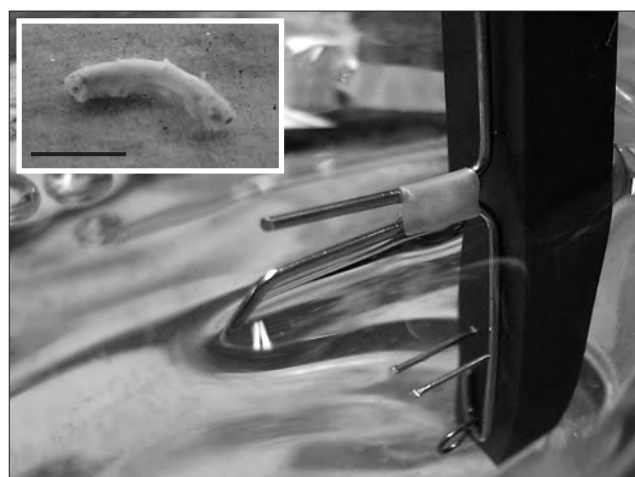
FIGURE 1 A typical mouse aorta section after careful cleaning for extraneous tissue (Insert), scale bar represents 4 mm, and once suspended and fully tensioned, as described in the materials and methods.
